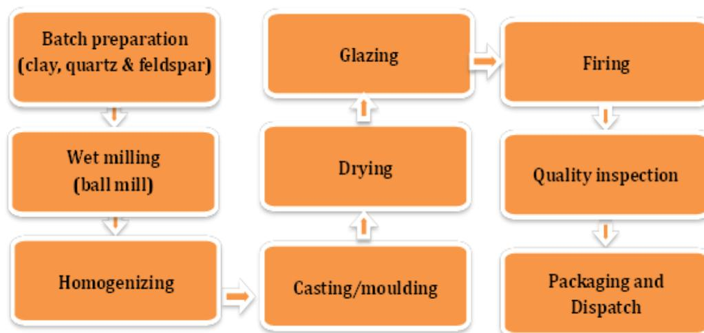
**Figure 2.3:** Manufacturing process of a typical ceramic unit
